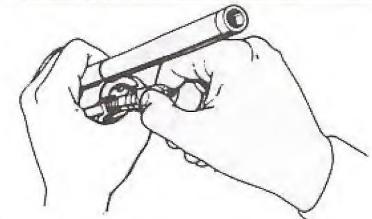
Insert the firing pin, firing pin spring, and locking piece into the bolt head carrier. Depress the locking piece into the carrier, and turn it one quarter turn clockwise.
